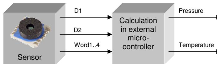
For both pressure and temperature measurement the same ADC is used (sigma delta converter):
